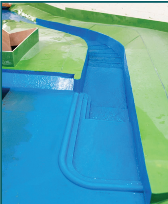
Photograph 1: 1:20 scale model of Roath Park spillway (bridge omitted from the model)
